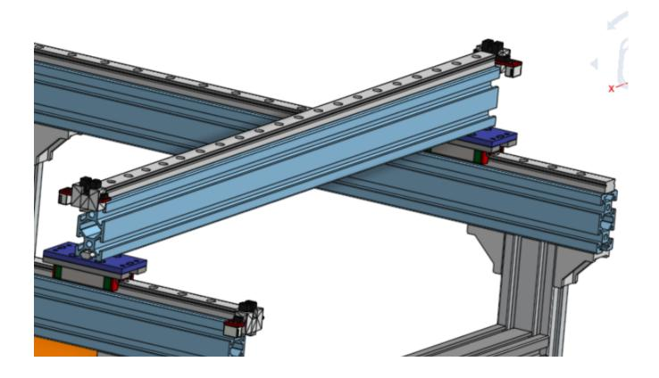
Lastly lets assemble the endstopsensorholder.stp and Optical Endstops end of the channels. 3D print the endstopsensorholder.stp x 4 pcs. Assemble them with the connector on the outside or facing to the back of the device. Having these on will prevent the sliders from coming off and the balls falling all over the place.
