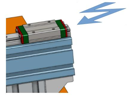
Then mount the bottom Sled block and screw it to the slide with 3mm screws.
