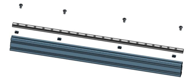
Next put the 12mm Rail Block (MGN 12) on the slide. Use caution because if the block goes off of the end of the slide, the bearings fall all over the floor..
