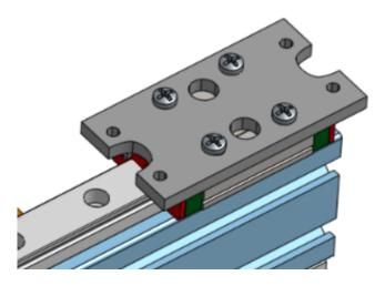
The next part is very clever but a little difficult to grasp. Attach the top sled block to the sliding cross rail with 3 x 8mm screws and T-nuts.
